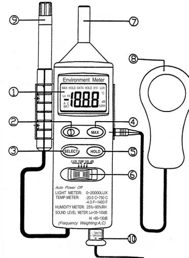
1. LCD display: 3 1/2 digits LCD display with units of Lux, x10 Lux, □, □, %RH, dB, A, C, Lo, Hi and low battery "BAT" MAX HOLD, DATA HOLD indication.
